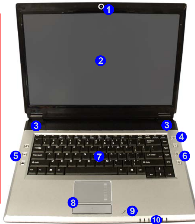
Figure 1 - 2 - Top View with LCD Panel Open Models A & B
